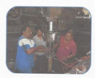
4.9 Press the pivot housing into position with help of hydraulic jack which is part of fixture. Pressure during mounting should not exceed 60 kN.
